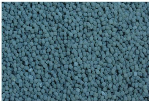
(a) \text{CaCO}_3/\text{PP} 共混包粘 (115 ^\circ\text{C} )
